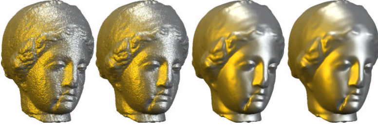
FIG. 3.2. From left to right we have depicted four different scale steps of the anisotropic geometric evolution of the Venus head. The surface representation was obtained by a laser scan with additionally added noise.
